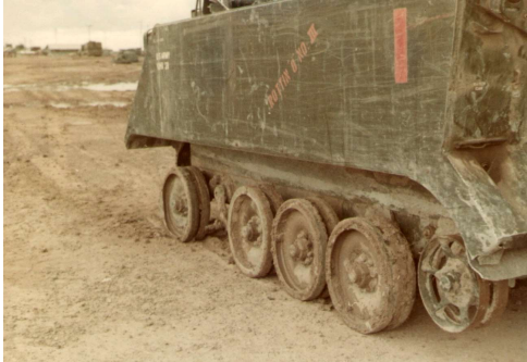
77 broken track.jpg | Track hit mine when Sgt. Haverkamp on way to R&R. (1284x895)
